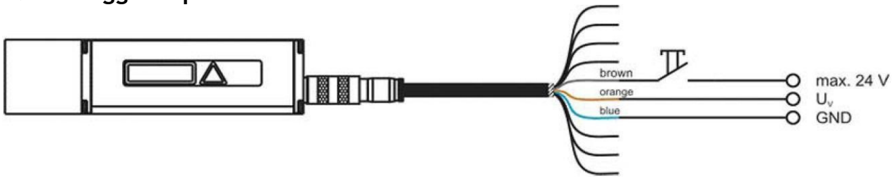
Figure 21: Wiring diagram of trigger input
