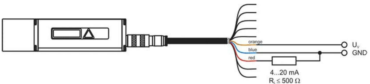
Figure 19: Wiring diagram of analog output
