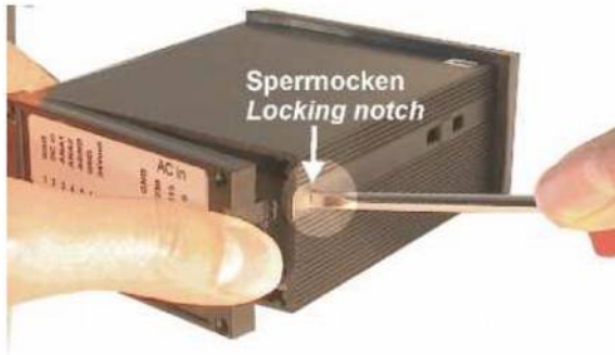
Removal of the back plane
