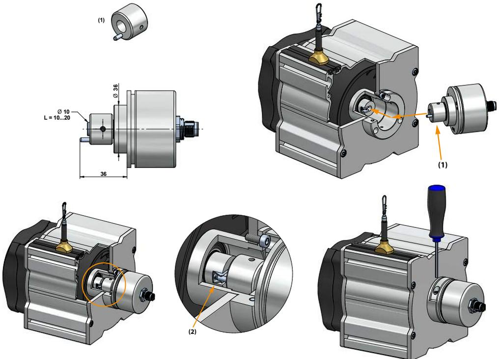
2. By tightening (1.5 Nm) the radial screw the encoder will be clamped and secured from twisting. Use a hexagon screwdriver, size 3.
