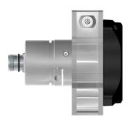
2. By tightening (approx. 2 Nm) the inner radial screw with a hexagon screwdriver, size 2.5 the encoder shaft will be clamped to the sensor mechanics and is secured from twisting. By tightening (approx. 2 Nm) the outer radial screw with a hexagon screwdriver, size 2.5 the encoder housing will be clamped to the sensor housing and is secured from twisting. The system is now ready to be mounted at the designated place.
