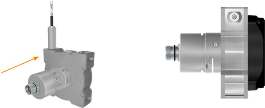
2. By tightening (approx. 2 Nm) the inner radial screw with a hexagon screwdriver, size 2.5 the encoder shaft will be clamped to the sensor mechanics and is secured from twisting. By tightening (approx. 2 Nm) the outer radial screw with a hexagon screwdriver, size 2.5 the encoder housing will be clamped to the sensor housing and is secured from twisting. The system is now ready to be mounted at the designated place.
