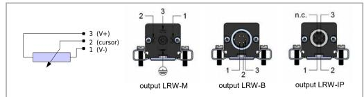
Sensor is to be used as voltage divider, using a maximum cursor current of  $Ic \le 0.1 \ \mu A$  (do NOT use the sensor as variable resistance!). Please pay attention to the notes on the last page.
